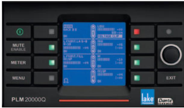
The front panel is the “local control center” for the PLM 20000Q. An intuitive, menu driven interface allows quick access to key functions using the moisture resistant silicone touchpad. Information is clearly displayed on the daylight-readable, 2.5-inch LCD panel. The soft-button keypad and precision rotary encoder provide control of processing and amplification functions, with key lock available.
